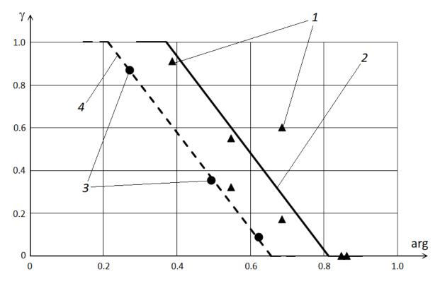
1 - starting material; 2 is the regression line for the source material; 3 - crushing products; 4 - regression line for products
